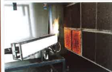
A1) The 750 C° heat of the radiant panel sets the coating film on fire.
