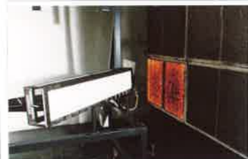
A1) Test start on MDF coated with a normal polyurethane cycle.
