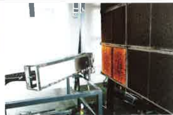
B2) The combustion sets off but the flame propagation speed is greatly reduced by the fire retardant coating.
