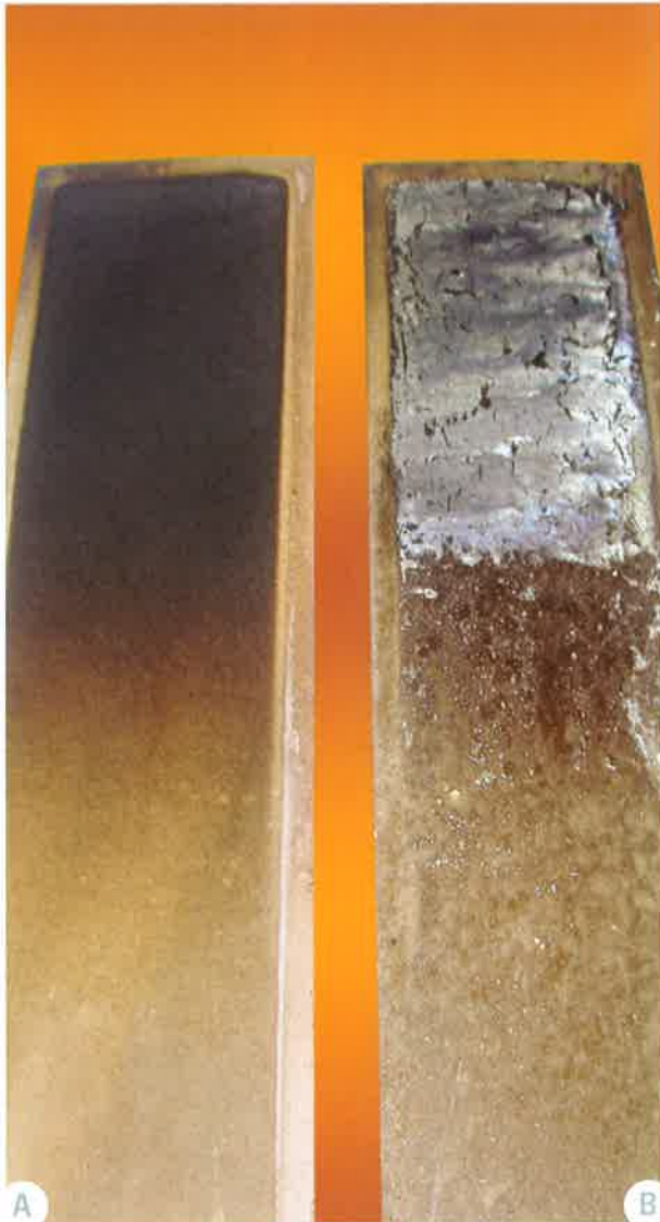
Comparison between fire retardant (A) and intumescent (B) cycle
