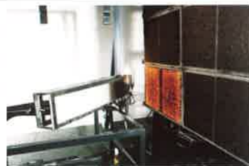
B1) Even if only partly damaged, the reaction that reduces the combustion speed is evident on the panel.
